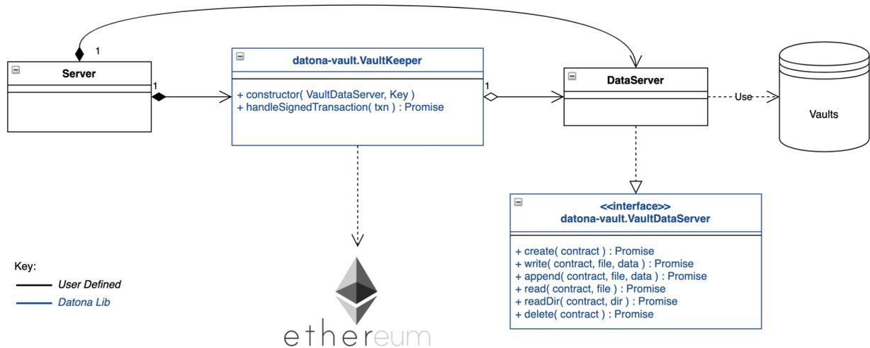
The diagram above shows the class relationships between the user-defined classes in black and the datona-lib classes in blue. The user-defined `DataServer` class must implement the `VaultDataServer` interface and promise to handle the 4 types of data request. All permission checks will have already been performed by the `VaultKeeper` so the `DataServer` need only perform the requests unconditionally.
